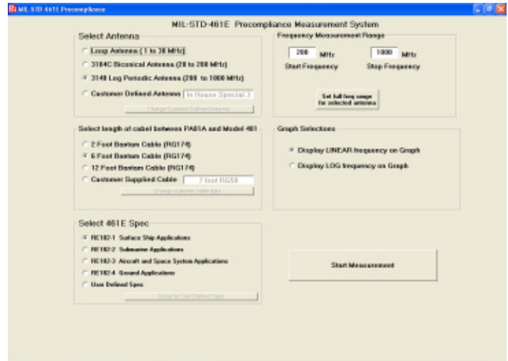
EMC-461 Measurement setup screen assures ease of use with simple selection of antenna type, cable length, desired specification limit, and log or linear frequency display.
